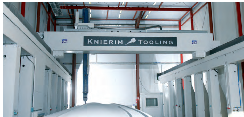
One of KNIERIM's three customized 5-axis milling machines fine cutting a rotor blade plug
